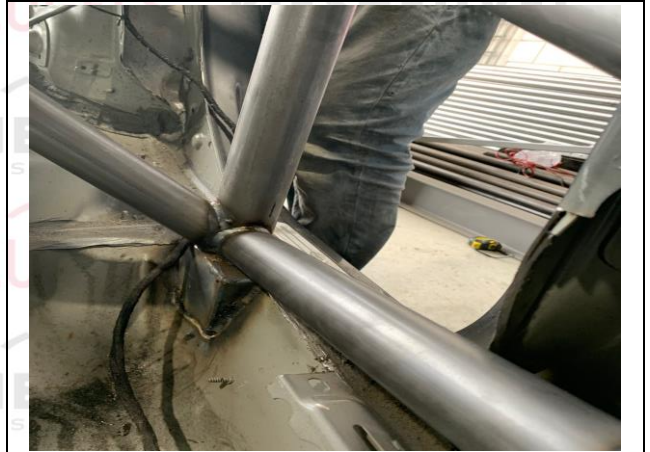
PHOTO 4 MAIN ROLLBAR TO FLOOR ATTACHMENT
