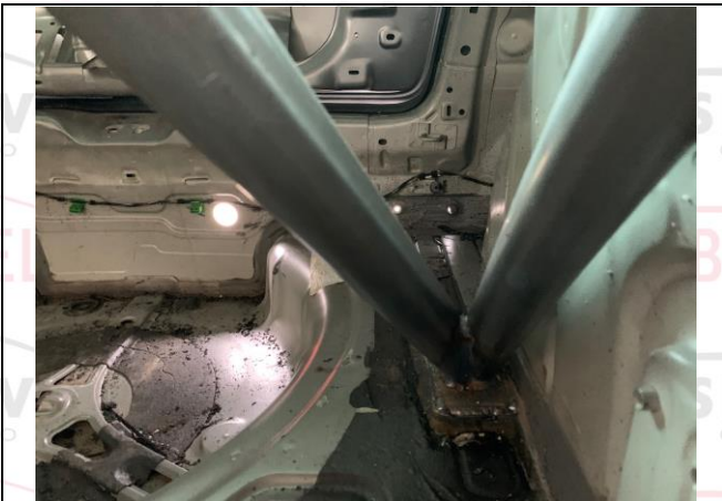
PHOTO 5 REAR BACKSTAY TO BODYSHELL ATTACHMENT
